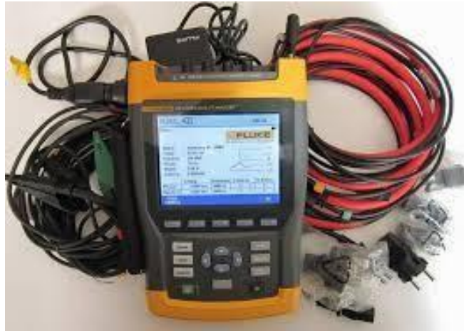
Fig 2: FLUKE 434-II POWER ANALYZER
